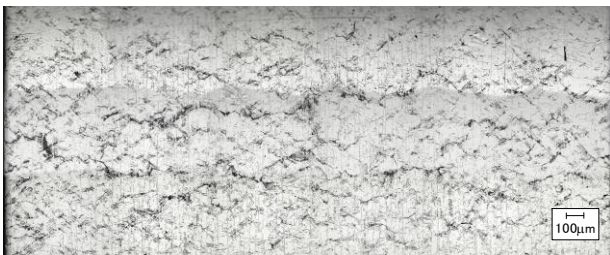
Fig.7 Observation of small crack growth path
